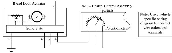
Turn ignition switch off, plug in connector, and turn ignition switch back to run position. While back probing actuator connector pins, check:
