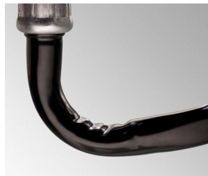
Inferior bend reduces coolant flow.
